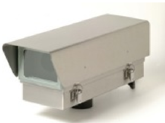
Figure 10. Commercially available diode-based luminance photometer: Hagner TLS-420.
