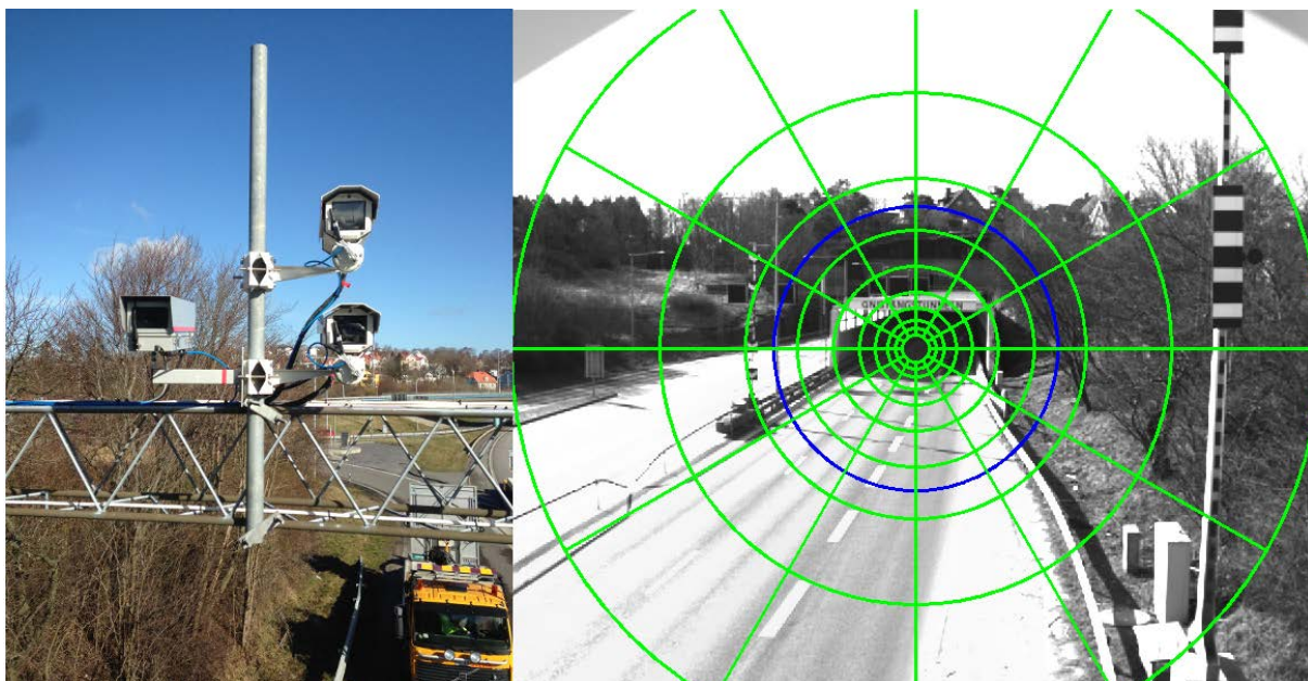
Figure 9. CIE 88 installation: Prototypes (left) and L_{seq} and L_{20} diagrams (right).
