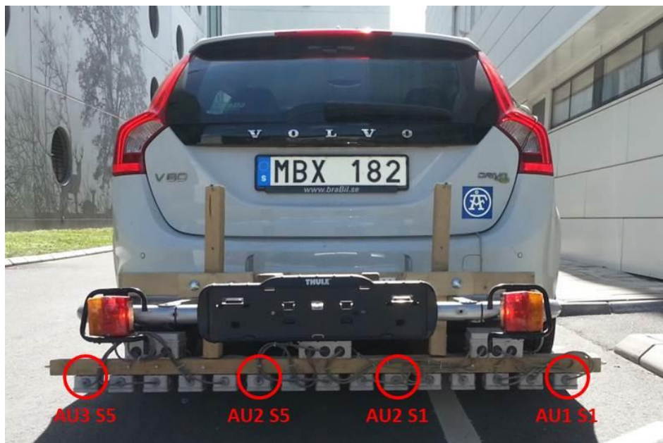
Figure 3: Test rig used for magnetic background noise measurements
