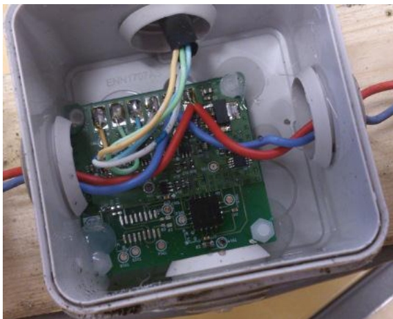
Figure 15 The sensor module, the sensor chip is in the lower right corner of the PCB
