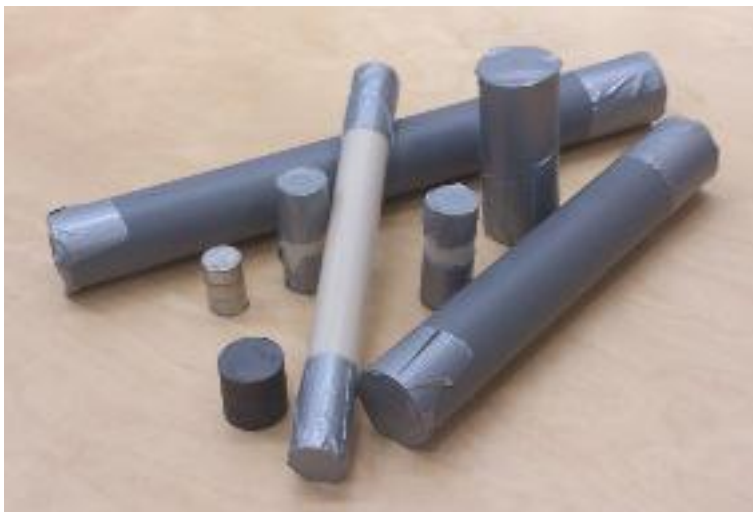
Figure 17 A selection of "magnetic pipes"; two 6 cm and one 24 cm white pipe for neodymium magnets and 10 cm, 25 cm and 35 cm long pipes for ferrite magnets. A 3 cm neodymium magnet and a 3 cm ferrite magnet are included to the left for reference.
