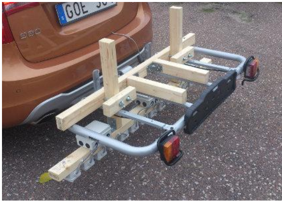
Figure 14 The sensor system mounted on the test vehicle's tow ball, with the sensor array seen in the smaller grey boxes beneath the beam holding the acquisition units. The grey cable from the trunk is the power supply to the system and the CAN bus.
