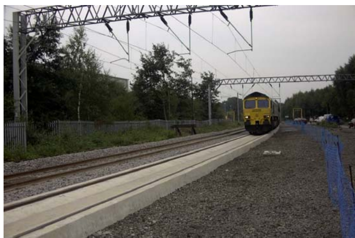
Figure 8 Embedded Rail System (BBERS)
