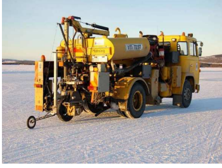
Figure 8: The mobile tire tester B12 operated by VTI
